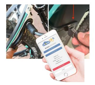
If you want to stop and park somewhere temporarily, the user can lock the bike using the application by clicking LOCK and pulling the handle down until there's a click sound. It unlocks by clicking the UNLOCK with the application. After using the bike, the user must lock the bike on the station using the application.
